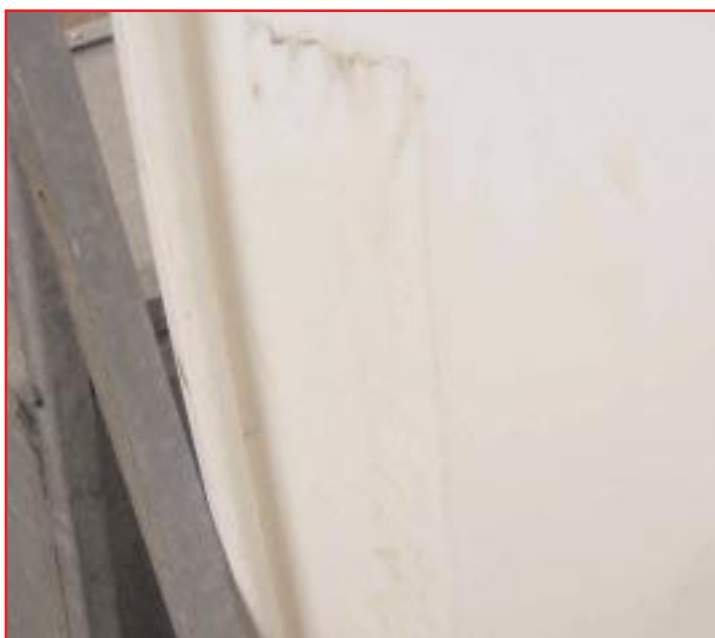
DUCT TAPE STUCK ON THE SIDES OF THE NEW OPPIES NEEDED SPECIAL CHEMICALS TO REMOVE IT AND IT MARKED THE HULL.
